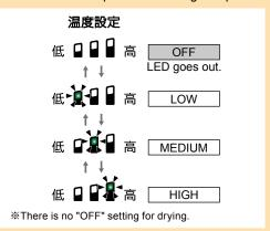
If the button is not pressed for about 10 seconds, the temperature adjustment LED will go off, but the setting will be retained.
