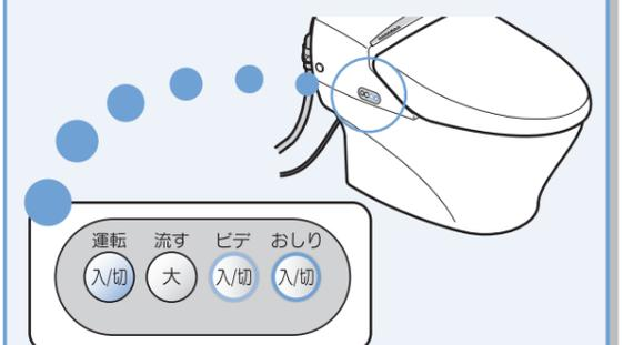
※Use these buttons if the batteries of the remote control are dead.
