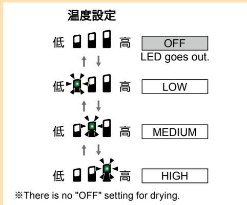
If the button is not pressed for about 10 seconds, the temperature adjustment LED will go off, but the setting will be retained.
